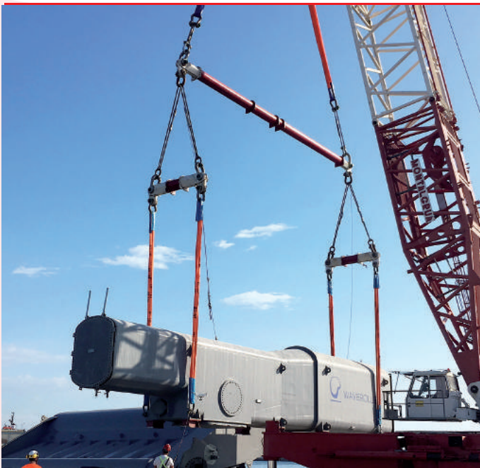
Textile slings: round, flat, multi-leg, made-to-measure from 500 kg to 600 tonnes and more
