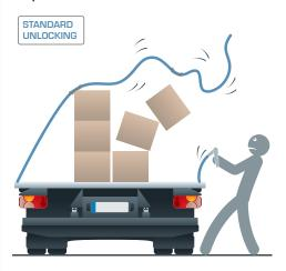
Before removing the bracing to unload, it is essential to check the stability of the load in order to prevent accidents.
