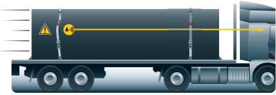
During the transport, the lashing systems lose tension (road degradation, emergency braking).
