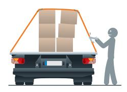
The tensioner's gradual notch by notch release makes it possible to make unloading safer and to adjust its stability when necessary.
