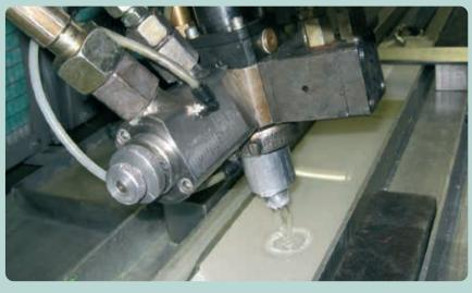
M Production process of a double side POLYSAFE polyurethane sleeve.
