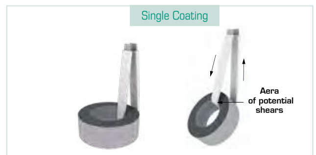
In the case of lifting without a sliding polyurethane sleeve, the risk of tearing and damage is much greater (see tear zone, diagram above left).
