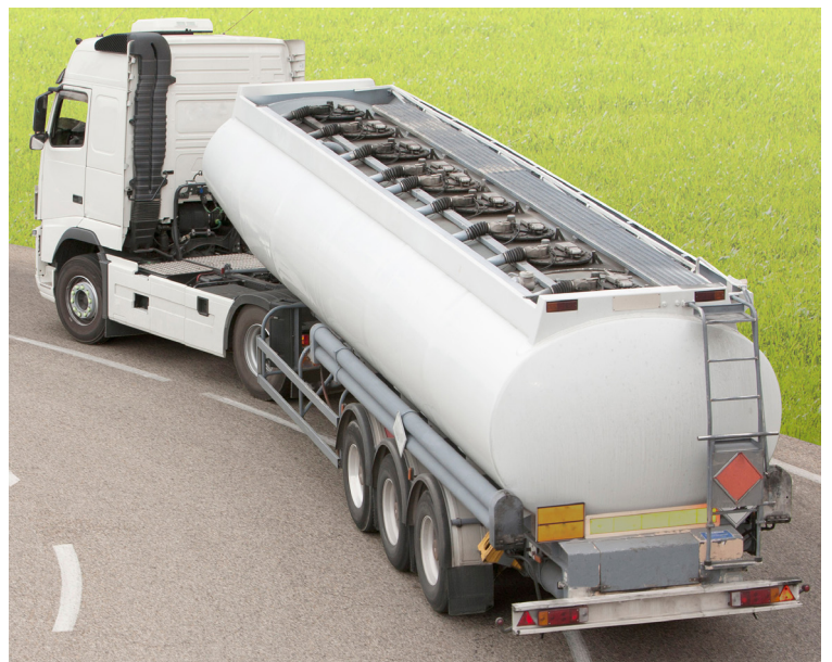
Tank lorry with platform requiring the use of a harness
