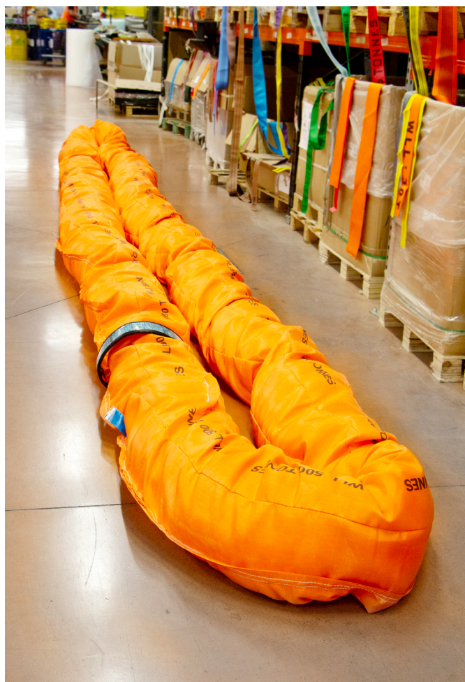
Round sling - 500 tons, 7 meters (manufactured in our workshop in Rang - department 25)
