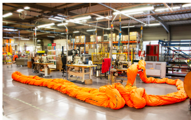
Round sling - 400 tons, 15 meters (manufactured in our workshop in Rang - department 25)
