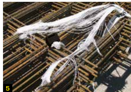
4 It is impossible to remove the sling without destroying it, making it unusable.
