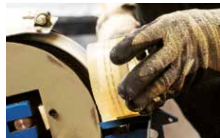
Sanding of a polyurethane-coated webbing.
